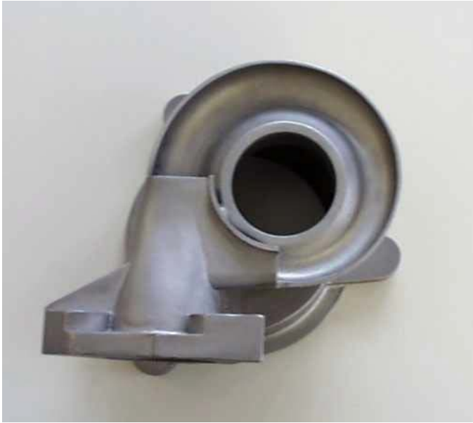
Figure 6: Cross-section of a precision cast turbine housing
