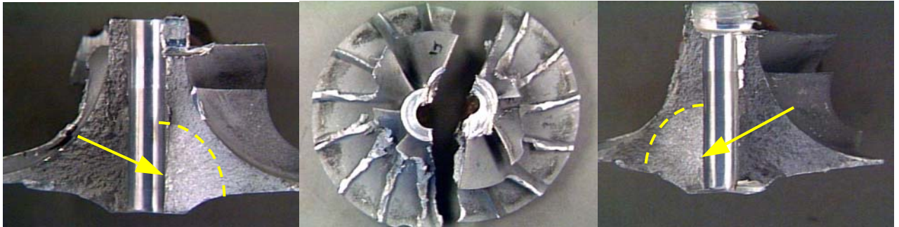
Figure 1: Classic type of LCF hub burst
