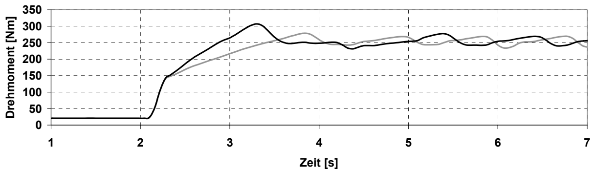
Figure 7: Simulation of the build-up of the charging pressure and torque for a load surge at 2000 rpm
