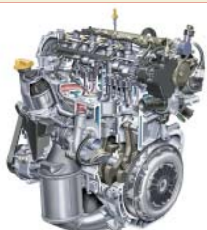
The compact 1.3 liter (80 cubic inch) common-rail diesel is the heart of an entire generation of Opel, Fiat and Lancia models.
