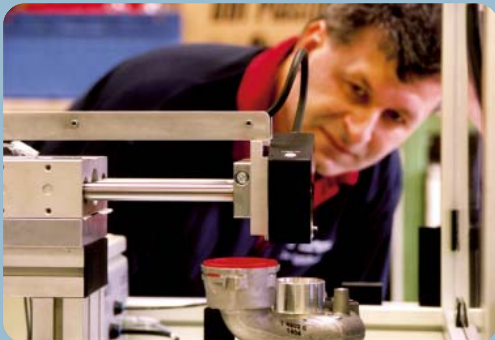
The components were checked and measured using cameras and laser technology.
