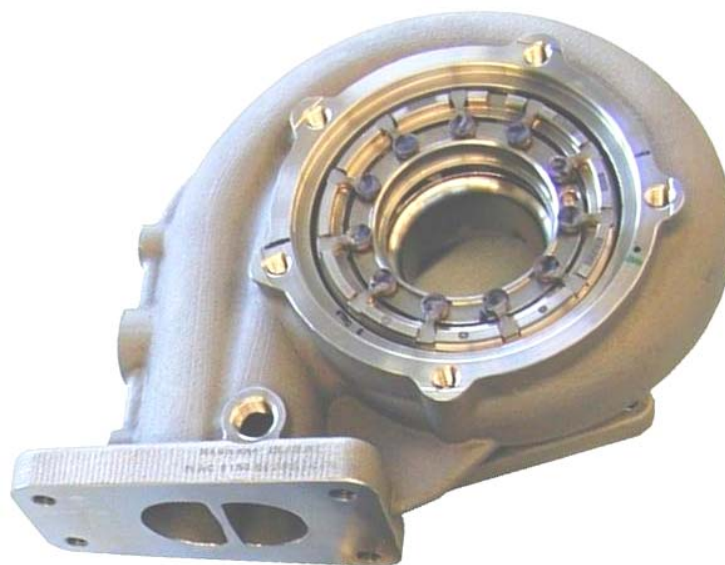
Figure 3.2.3: View through dual-volute turbine housing with VTG guide vanes
